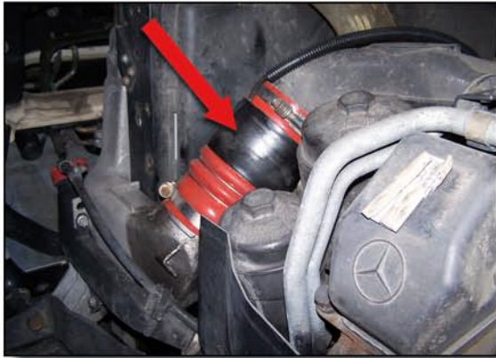
Pre-fabricated charge air hose manufactured with a coil system, replaced Mercedes Benz Part-No. A 003 094 08 82
