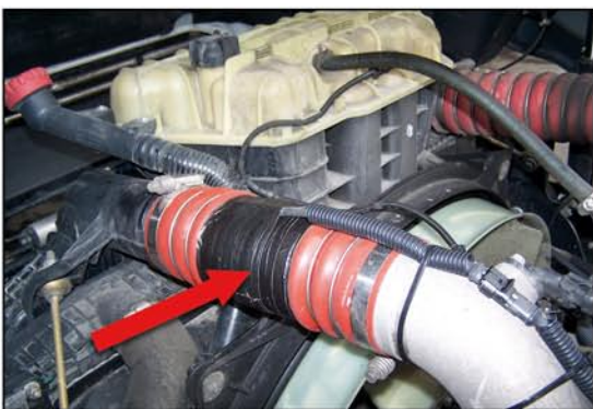
Pre-fabricated charge air hose manufactured with a coil system, replaced MAN-Part-No. 81.96.301.0900
